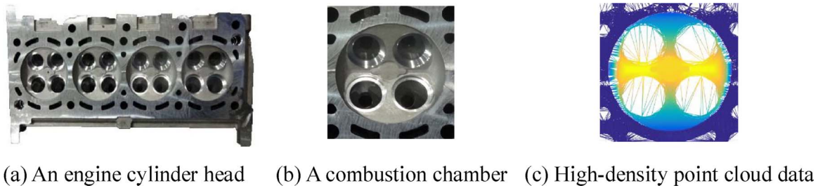
Fig. 1. The high-density point cloud data of a curved surface of an engine cylinder head.
